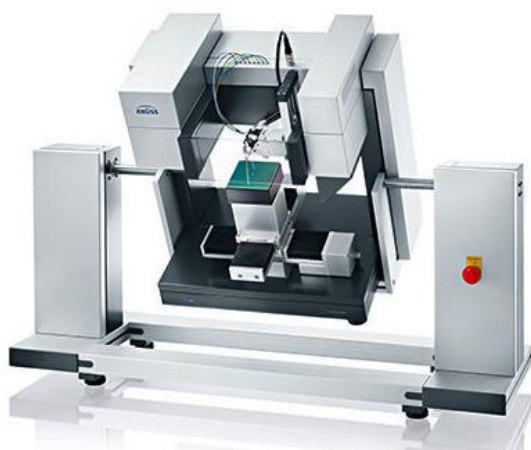
Fig. 4. Drop Shape Analysis System DSA100E (Krüss GmbH, Germany) for surface wetting studies with a tilting table, a dosing system, a temperature control cell, a surface rheology, and a foaming module
