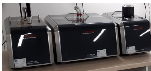
Fig. 7. Laser Diffraction System Analysette 22 NanoTec (Fritsch GmbH, Germany)
