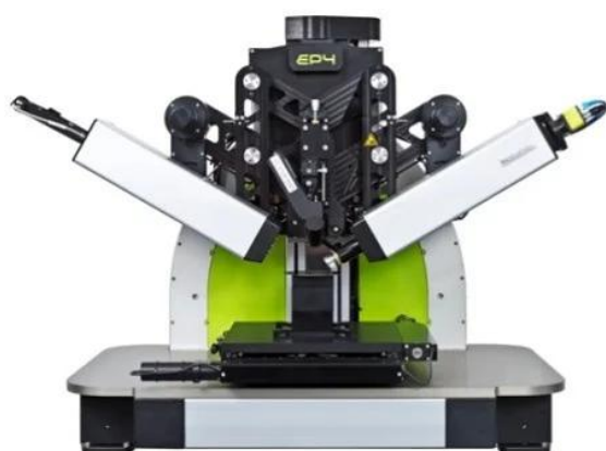
Fig. 2. Imaging ellipsometer EP4 (Accurion, Germany) used for per-pixel \psi/\Delta mapping and thin-film thickness retrieval
