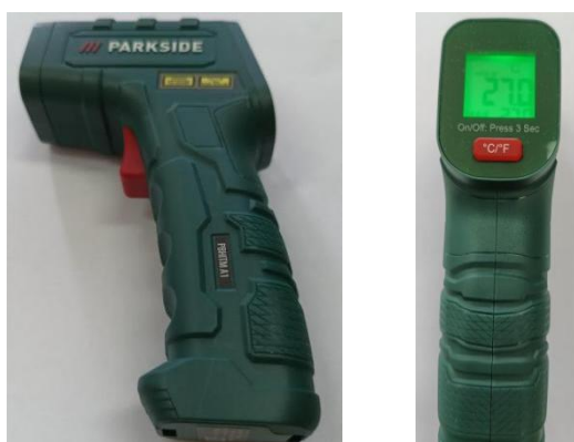
Figure 4. Example of a commercially available infrared thermometer used in the calibration process
