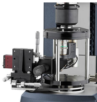
Fig. 1. Optical attachment mounted on a TA Instruments rheometer, enabling in-situ imaging during shear and oscillatory tests on a temperature-controlled plate-plate geometry
