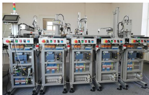
Fig. 2. Modular assembly system.
