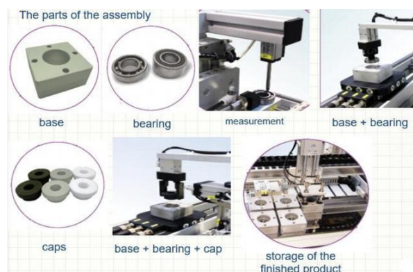
Fig. 1. Parts of the assembling process.
