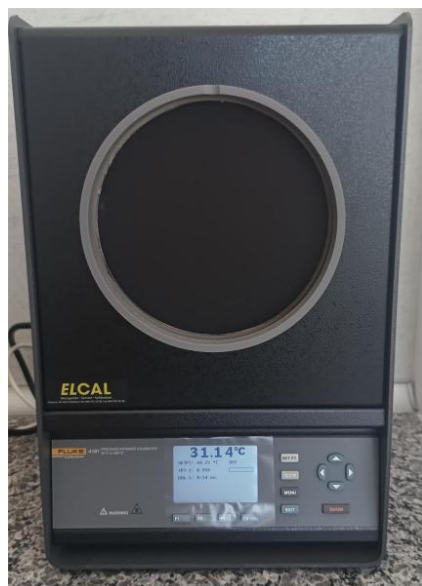
Figure 3. View of the Fluke 4181 infrared calibrator employed at the Center of Competence, Technical University – Gabrovo
