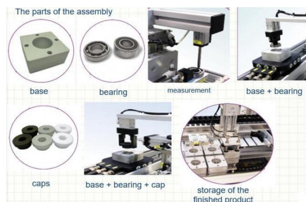
Fig. 2. Parts of the assembling process.
